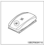
(1) This switch is used for operation of the fan on the overhead guard.
